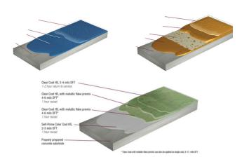
50 Marketing developed layered concrete coating cutaway illustrations and animated views for **Flexmar's** coating systems.
